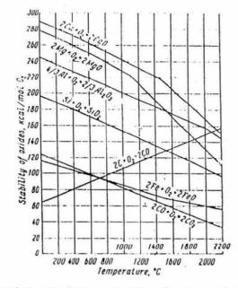
Fig. 1 . Relationship between stability of oxides and temperature
