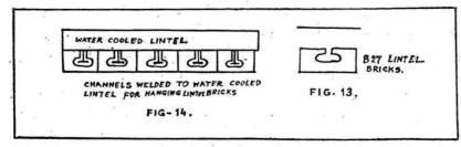
Fig. 13. Fireclay shapes used for lintel Fig. 14. Fireclay shapes with welded channels
