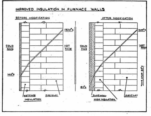
Fig. 5 Modified wall insulation.
