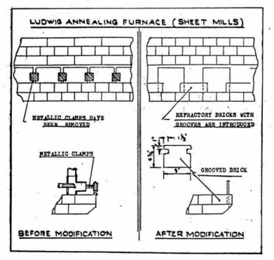
Fig. 4 Replacement of stainless steel holder by grooved brick.
