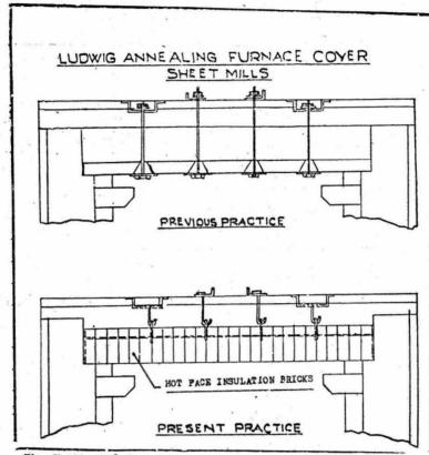
Fig. 3 Modification of furnanace cover by replacing refractory tiles with hot face insulation.
