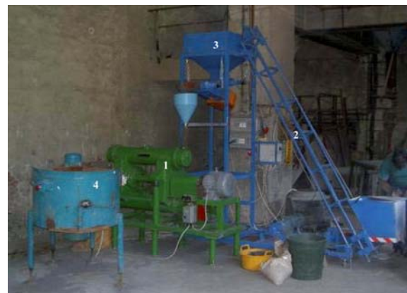
Figure 10. Equipment used in pilot scale experiments 1) 20 U PALLA vibration mill, 2) bucket elevator, 3) Vibration feeder, 4) Turbo-mixer
