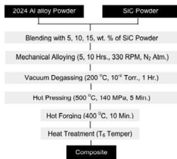
Figure 1. Flow sheet for preparation of the 2024 P/M Al alloy SiC composites
