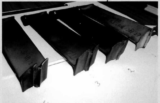
Photograph of Z-notch of tip shrouded portion of the LPTR blades where BZL welding have been carried out as marked by arrows
