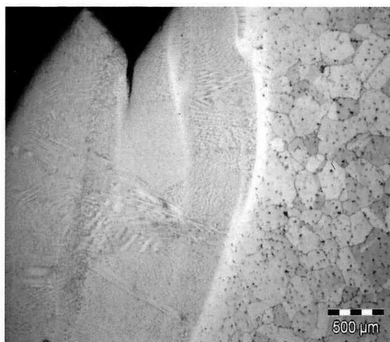
Fig. 6: Optical photograph showing BZL welding layers in case of 4 th time BZL welding
