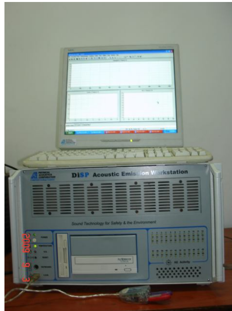
Fig. 6.2 A 32 channel Digital Image Signal Processing (DISP), acoustic emission system interfaced with a computer
