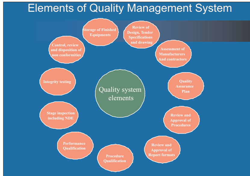
Fig. 3: Typical Quality Management System in Nuclear Industry
