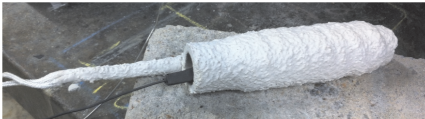
Fig. 1: Photograph of an EM sensor (length 140 mm, inner diameter 20 mm) designed for high temperature use, in this case monitoring phase transformation in a steel rod sample during air cooling from 1000°C.
