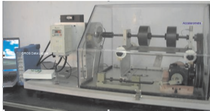
Fig. 3: Experimental Set up (Machinery Fault Simulator)
