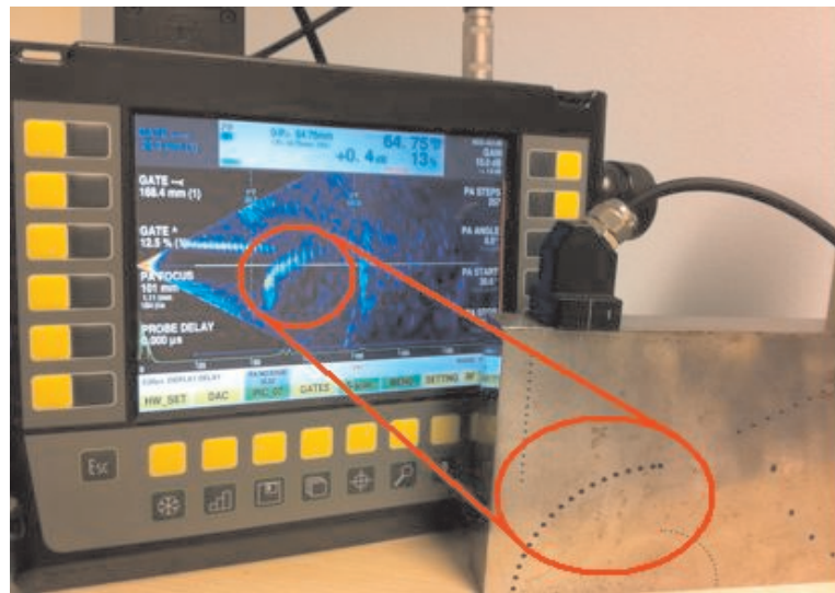
Fig. 4: Constructed system DIO1000, phased array - calibration gauge
