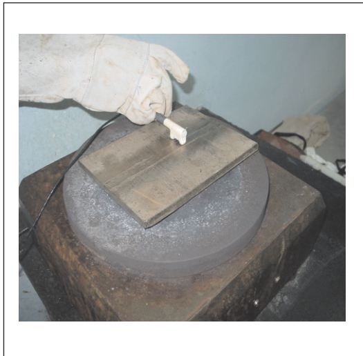
Fig. 12 (a) Scanning of the hot weld plate using high temperature ECT probe
