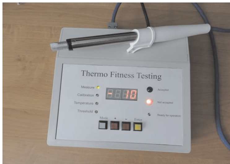
Fig. 12: Thermo Test Instrument for Manual Part Control
