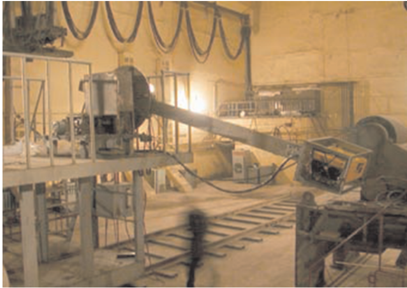
Fig. 16: 7.5 MeV Betatron Inspection Station in Volgogradneftemash production plant, Russia
