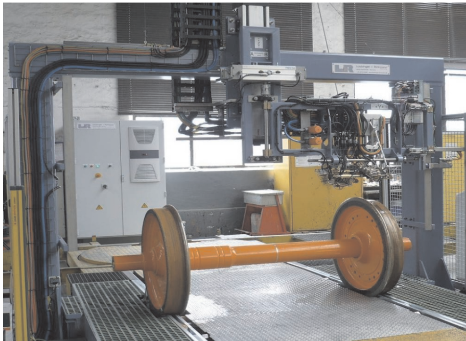
Fig. 2: Automated Railway Wheel Inspection (5)
