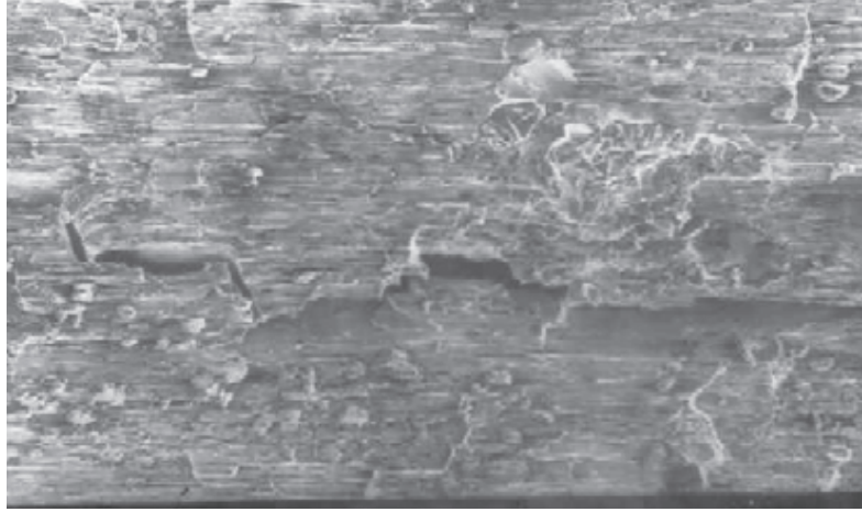
Fig. 5: Fractograph of the failed wire
