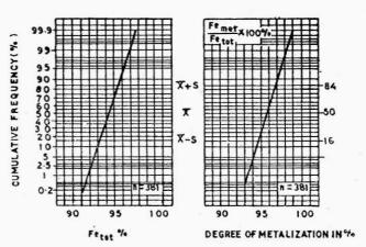
Fig. 9 Scattergram of Fe-contents and degree of metalization in metalized iron ore over 6 weeks of operation.
