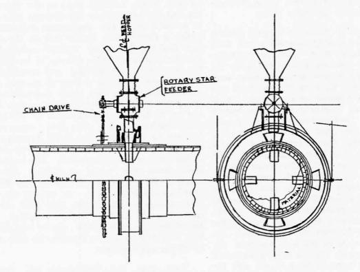
Fig. 2 Coal Throwing arrangement
