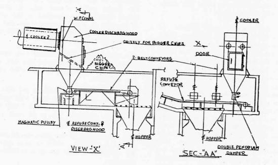
Fig 4 Cooler Discharge Arrangement
