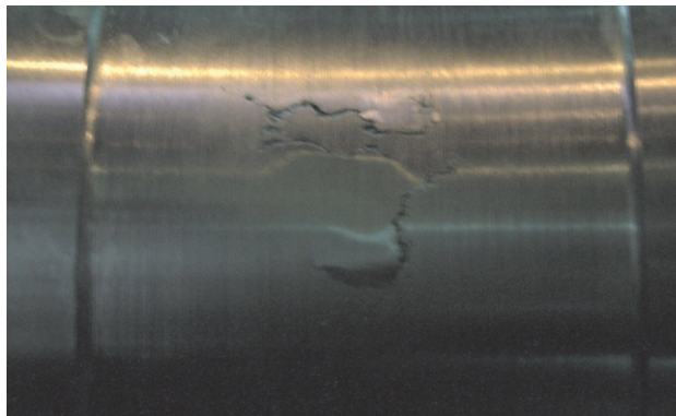
Fig. 1: Crack networks and spall occurred on the roll surface
