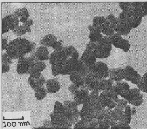
Fig. 10 : TEM image of AlN powder prepared at 1630°C
