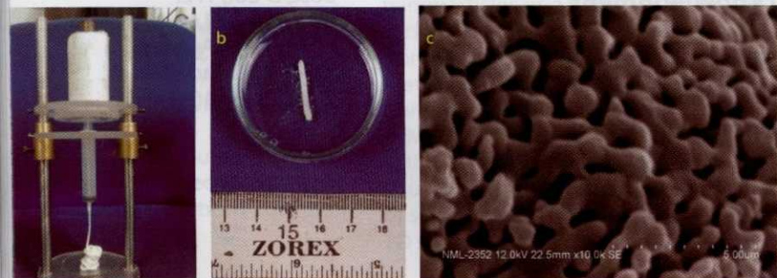
Fig.1: Injection of HA nanoparticles (a), water stability of self-setting nanoHA exhibiting bubble formation due to porous structure (b) and porosity confirmed by SEM studies (c).
