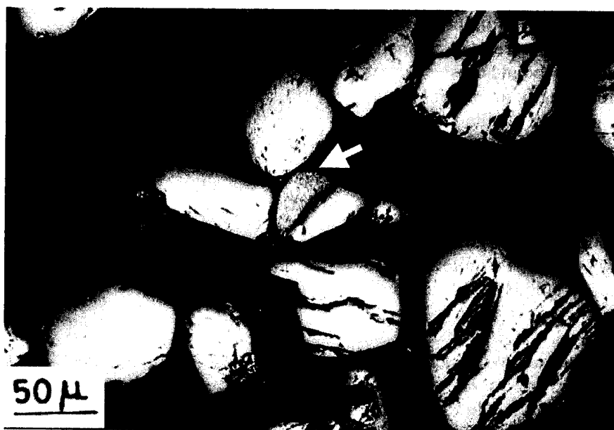
Fig.4b: Alteration of ilmenite grains (shown by arrow) from Navaladi
