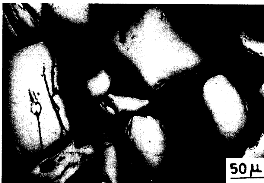
Fig.4a: Various shapes and sizes of ilmenite grains from Navaladi
