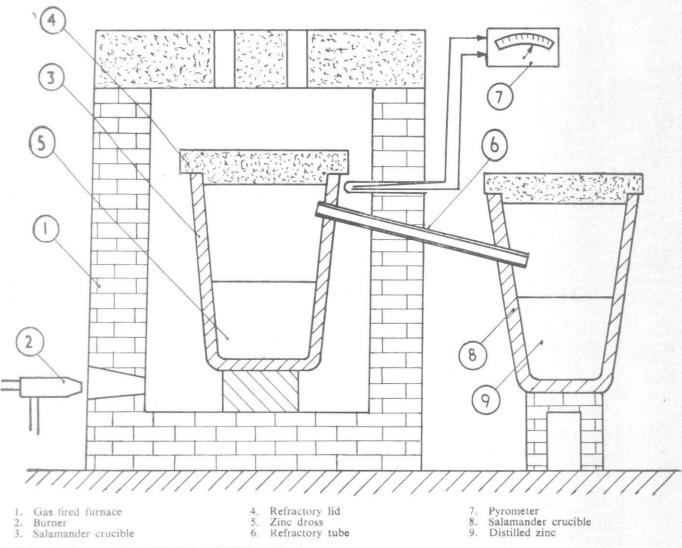
1 Schematic diagram of atmospheric zinc distillation unit
