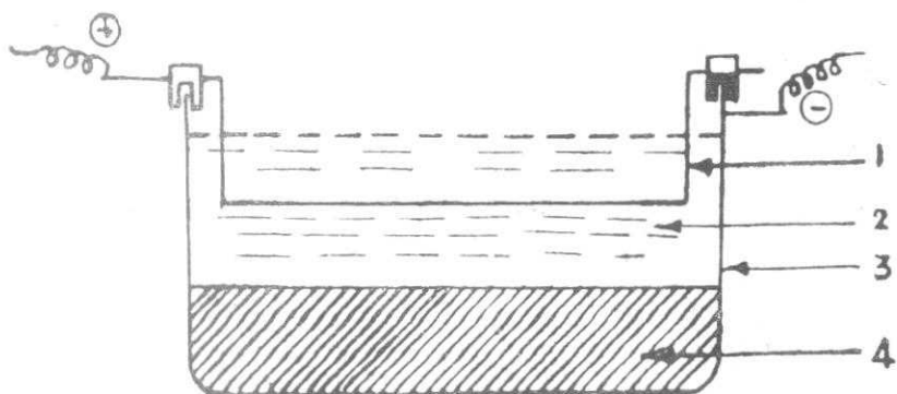
1 Schematic representation of the cell set up used for direct reduction of by-product compounds 1. Wire gauze anode 2. Electrolyte-alkali solution 3. Cell container cathode 4. Solid by-product compound
