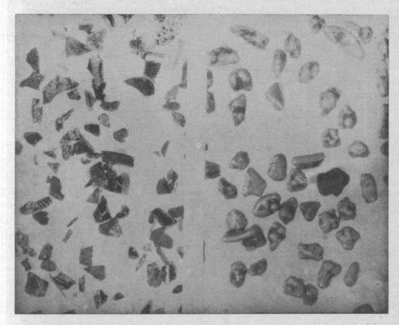
3A Iron particles making up the original fluidized bed
