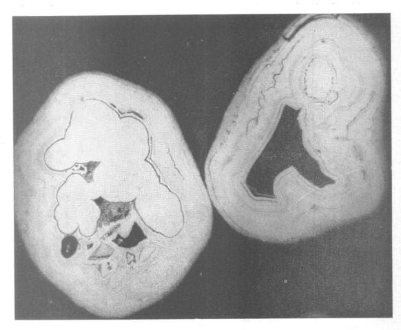
4 Enlarged cross-section of some of the particles showing layers of carbonyl iron built up during decomposition
