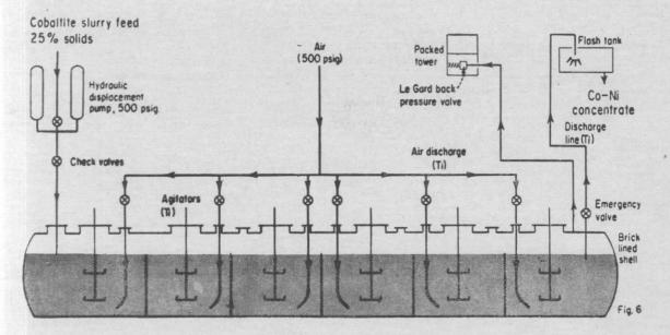
5 Sketch of the autoclave used in the Garfield Plant
