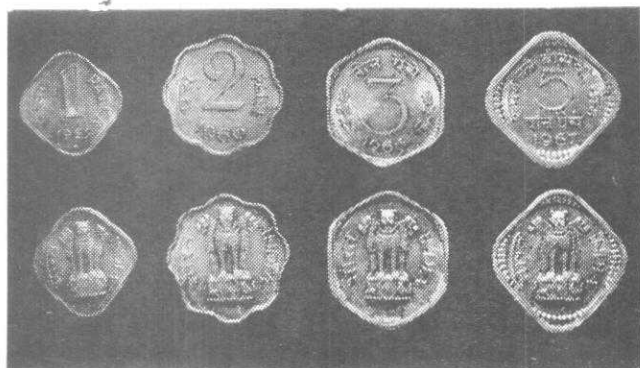
New 5, 3, 2 and 1 paisa coins made of Al-Mg alloy developed at National Metallurgical Laboratory and Government of India Mint, Bombay
