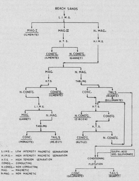
Fig. 4.1 General Flow Sheet for Treatment of Beach Sands
