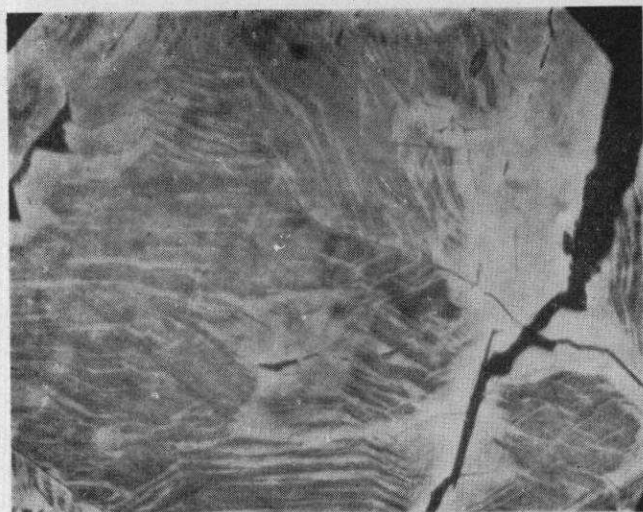
Fig. 3.8 Flame like aggregates of violarite (white) in Pyrrhotite (grey). Etched with KOH. X 168. Copper ore (Khetri, Rajasthan).
