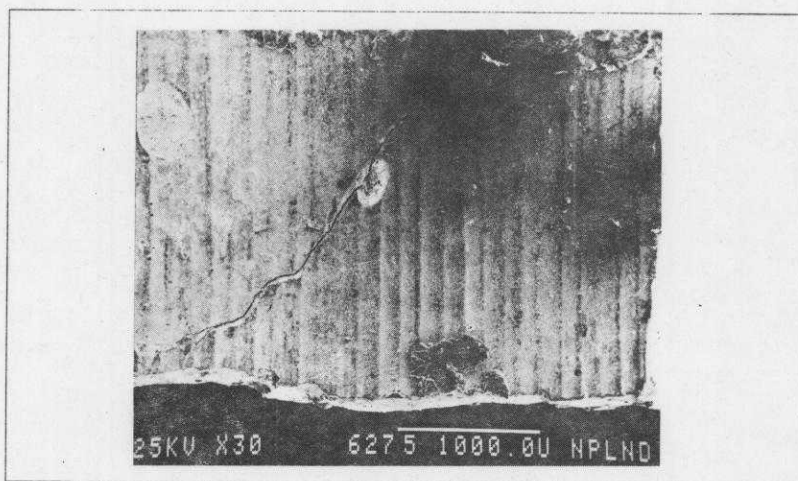
Fig. 6 : Electron micrograph showing circumferential cracks inside the surface
