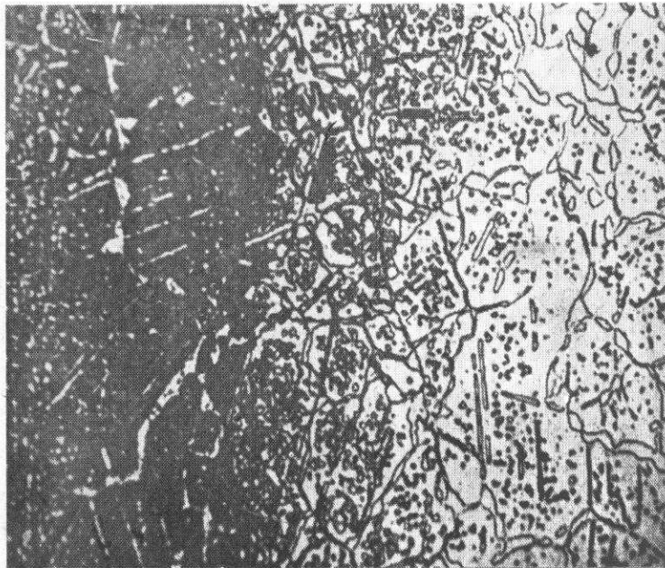
FIG. 6. Furnace Burner Shell Carburised during Service. Etched in Modified Marbles Reagent X-250. (After Payson and Savage 38 ).
