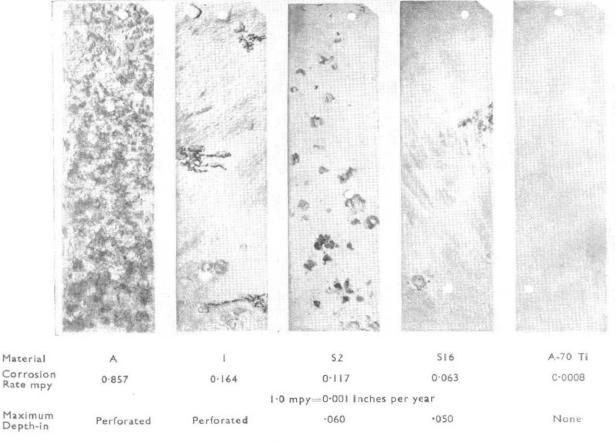
Fig. 7. Effects of flowing sea water (5 years at 3 feet/second) on several structural metals.
