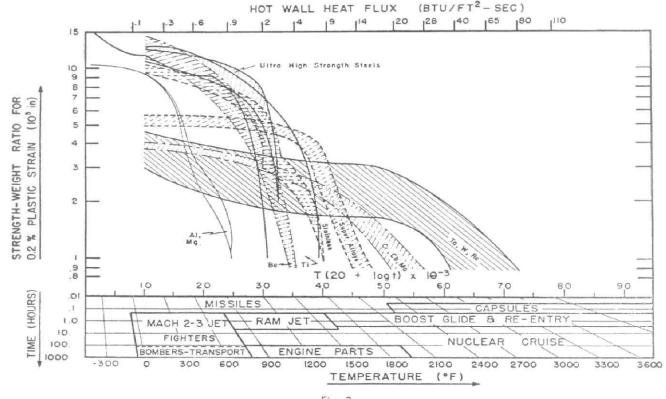
Fig. 2. Iso-plastic-strain diagram of materials used for advanced aerospace vehicles.
