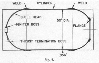
Typical rocket motor casing used in solid fuel rockets.
