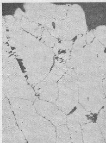
7b Stress 25 kg/mm 2 , rupture time 194 hrs.
