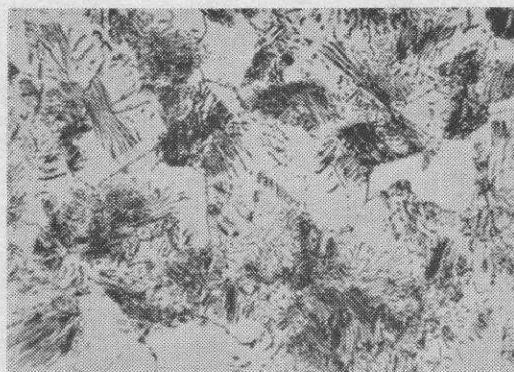
18 Heat no. B 2 -Aged at 800°C for 24 hours—oxalic electrolytic ×250
