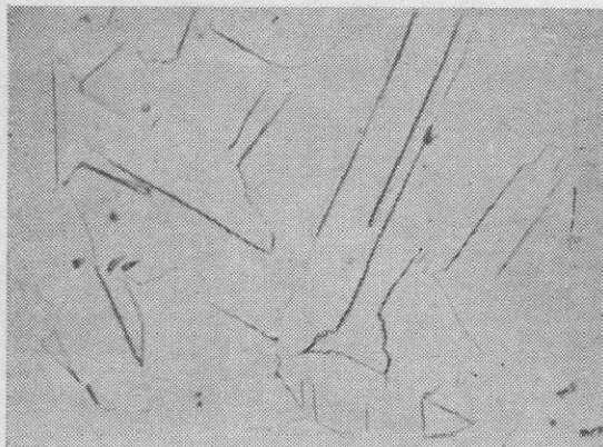
15 Heat no. B 2 -Aged at 400°C for 1000 hours—oxalic electrolytic ×450
