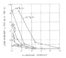
1 Effect of Cr and Al on oxidation resistance of Fe-Cr-Al alloys (From kornilov<sup>4</sup>)
