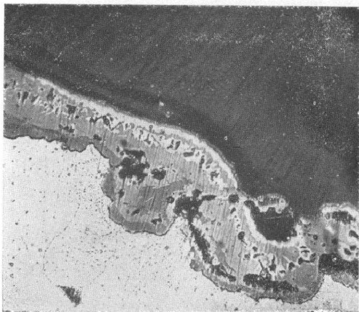
Fig. 6b. Scale formed at 950°C \times 500 .
