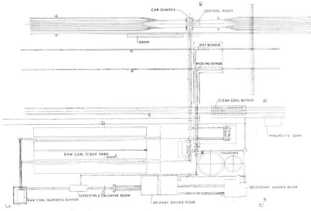
General arrangement plan of central coal washery at Dugda.
