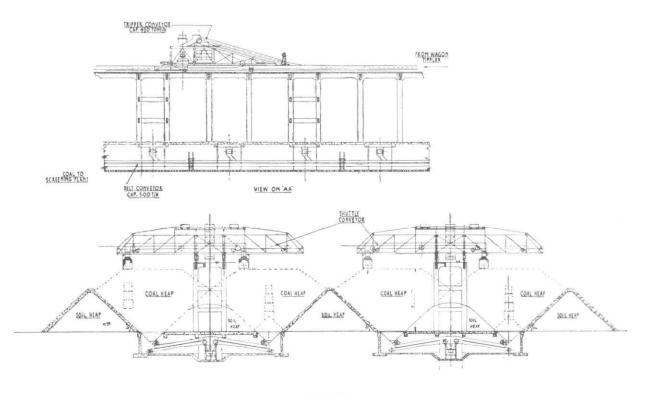
Arrangement of stacking and reclaiming in the ground storage.
