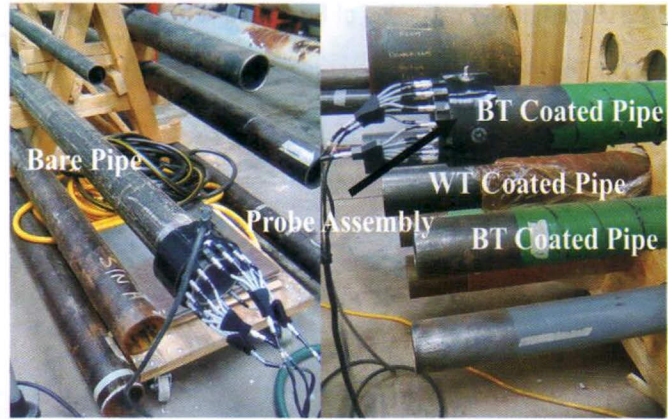
Fig. 6 : Photographs of tested bare and BT and WT coated pipes
