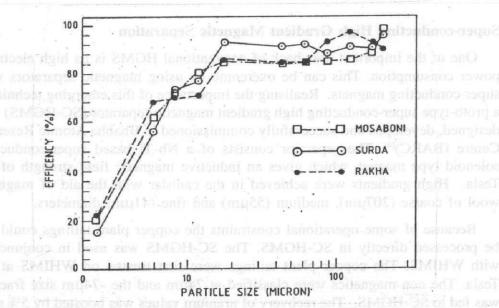
Fig. 4 : Efficiency on separation or uranium values in different size fractions of WHIMS concentrate of copper plant tailings
