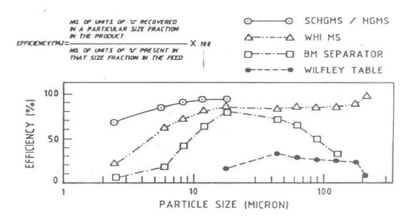
Fig. 6 : Comparison of the efficiencies of separation of uranium values in different size fractions in different gravity and magnetic separators (data on Mosabani copper plant tailings).
