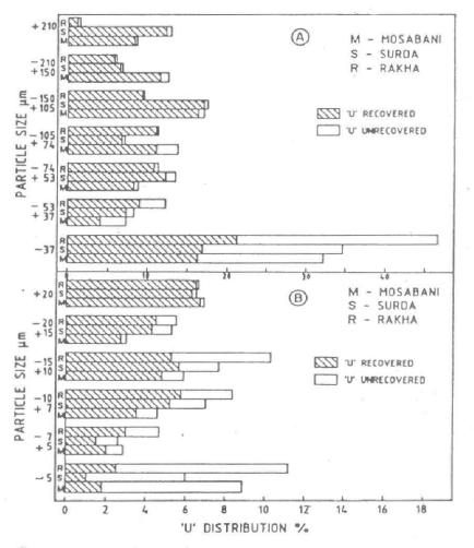
Fig. 3 : Recovery of uranium in different fractions of WHIMS magnetic concentrate of copper plant tailings. (A) Sizing on standard test sieves, (B), Subsieve analysis of -37 micron fraction on cyclosizer
