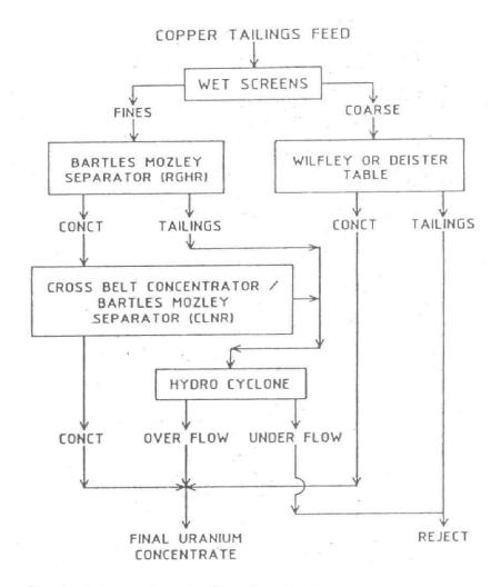
Fig. 2 : Integrated gravity flow-sheet for the preconcentration of uranium values from copper plant tailings
