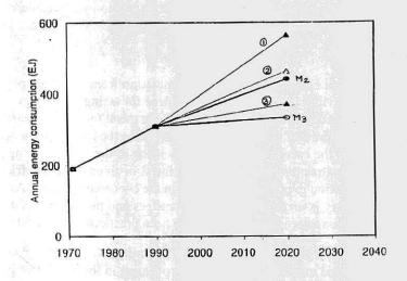
Fig. 1 : Three scenarios for aggregate world energy consumption upto 2020. The thin lines are for only energy efficiency case. The thick lines represent scenarios with both energy and materials efficiency improvement <sup>[1]</sup>.
