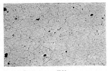
FIG. 2 — STRUCTURE OF K-MONEL AS SOLUTION TREATED AND AGED (  $\times$  300 )
