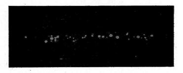
FIG. 5 — RADIOGRAPH OF UNSOUNDNESS IN MONEL ARC WELD RESULTING FROM USING DAMP ELECTRODES (  $\times 1$  )
