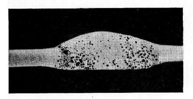
Fig. 8 (9534) — Macro-section of argon arc weld in Monel, using normal Monel as filler wire (  $\times$  10)
