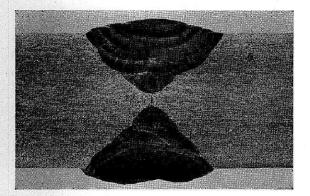
FIG. 7 (H. 2354) — MACRO-SECTION OF BUTT JOINT IN  $\frac{3}{4}$  IN. THICK MONEL PLATE. DOUBLE-VEE PRE-PARATION. LACK OF ROOT PENETRATION AT CENTRE OF JOINT (  $\times$  3)
