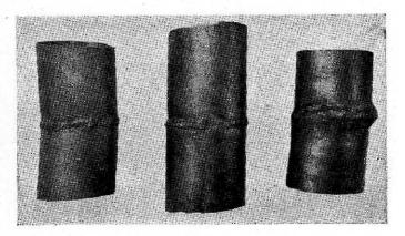
FIG. 19 — UNSOUND OXY-ACETYLENE WELDS IN MONEL TUBING, WHICH LED TO PITTING CORROSION  $(\times \frac{3}{4})$
