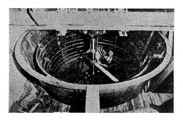
FIG. 4 — MONEL GRANULATING TANK FOR THE PRODUCTION OF POTASSIUM DICHROMATE (By courtesy of Chrome Chemicals Pty. Ltd., Parrametta, N.S.W.)
