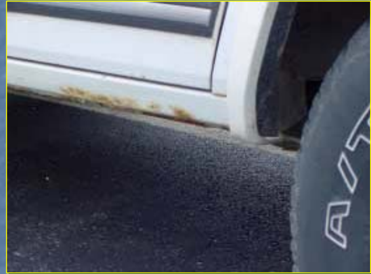
General corrosion of painted steel automobile body panel
