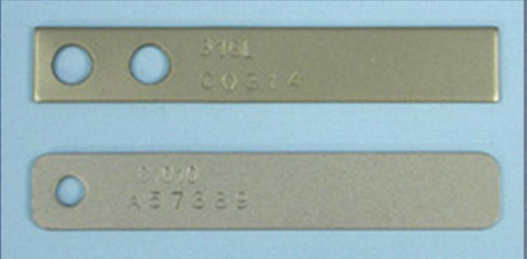
Flat test coupons that are used for corrosion testing
