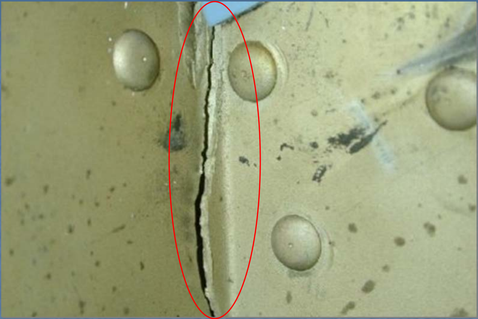
Stress corrosion cracking (SCC) of an aircraft component
