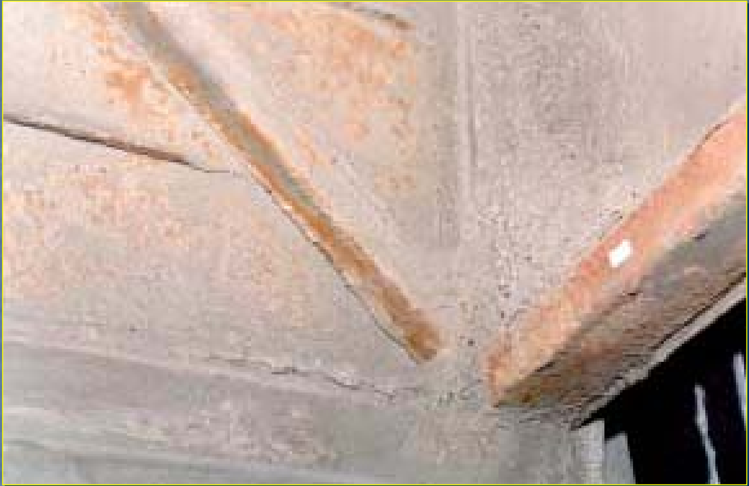
Photograph of poultice build-up of road contaminants in the wheel area of a bus
