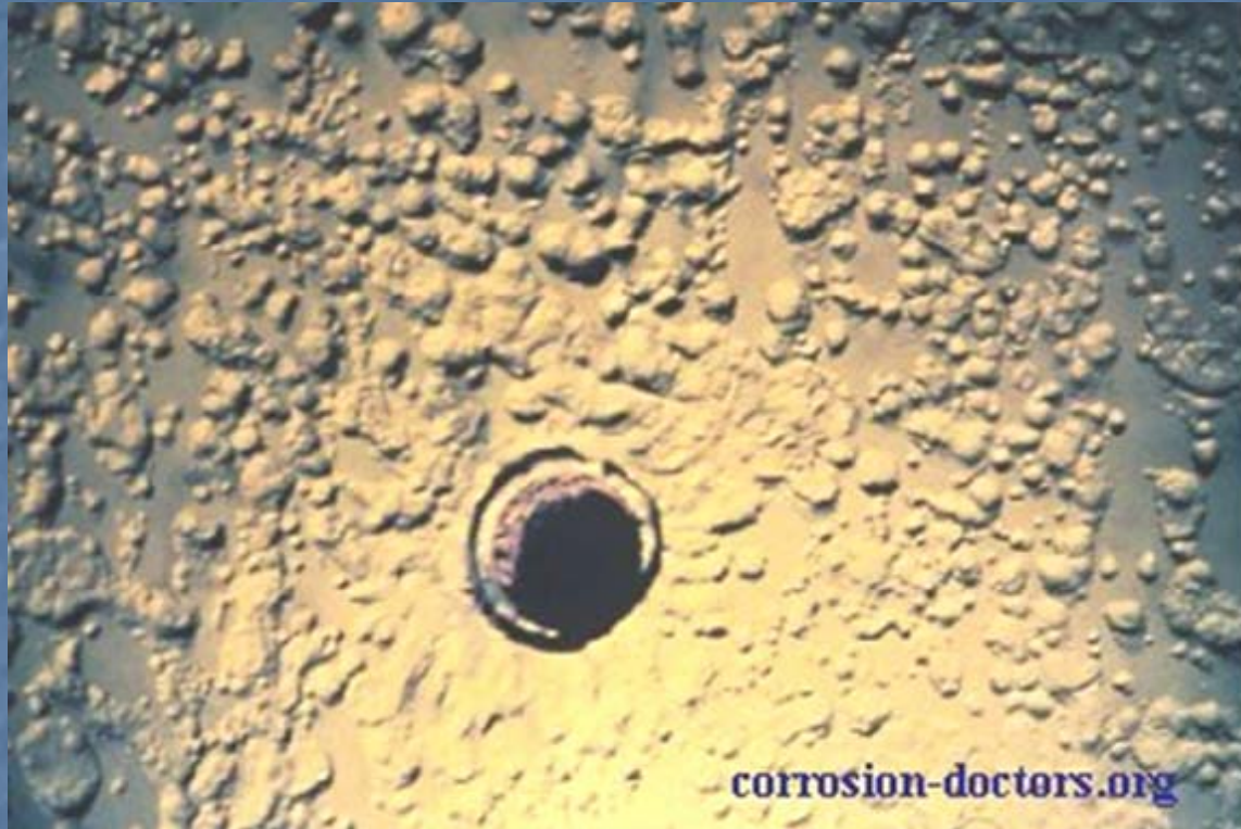
Cavitation corrosion of a deaerator
