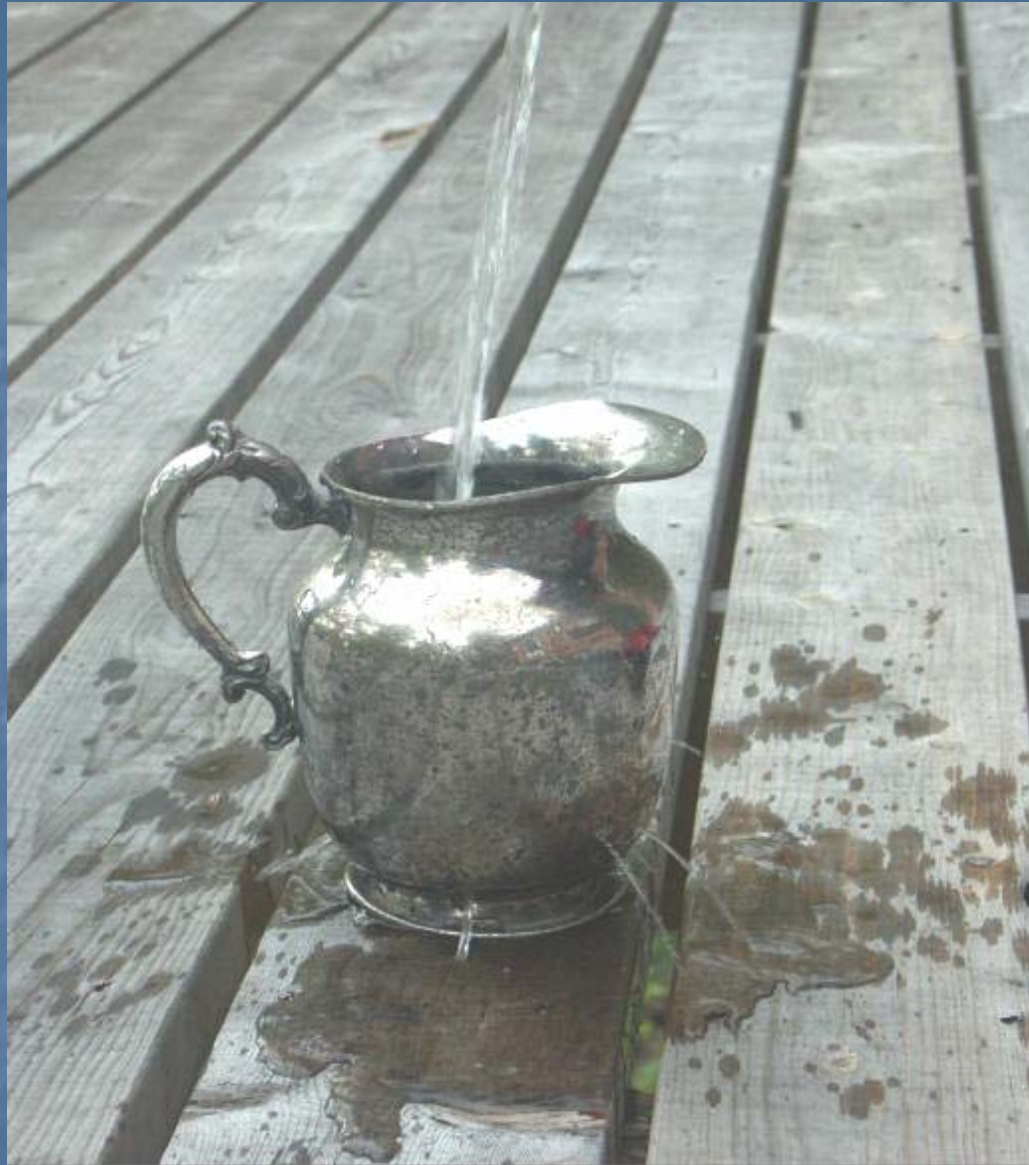
Pitting corrosion in a stainless steel water jug
