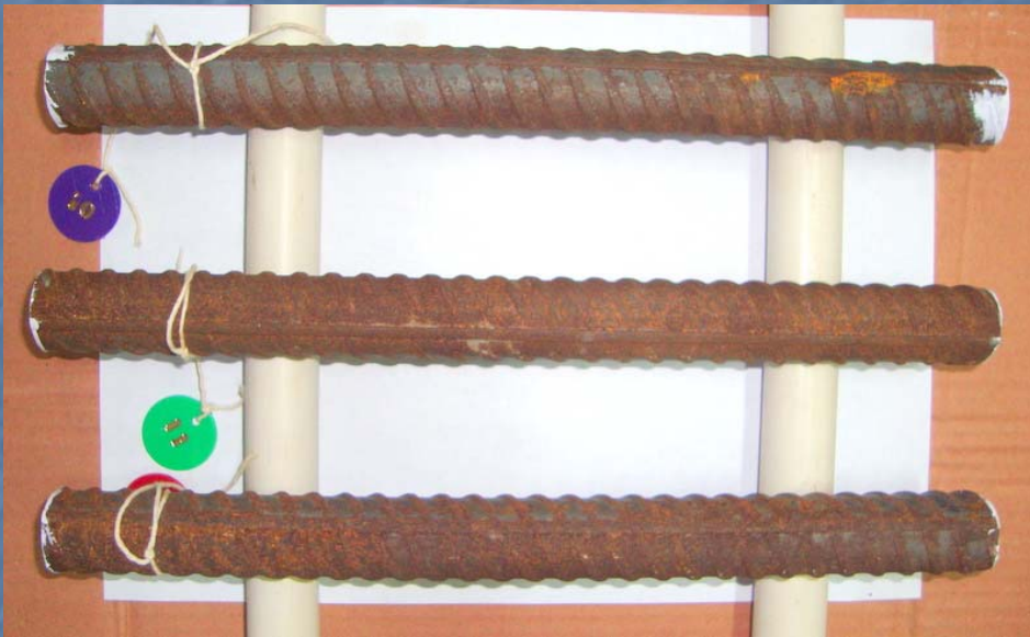
25 mm \varnothing TMT bar before NSS
