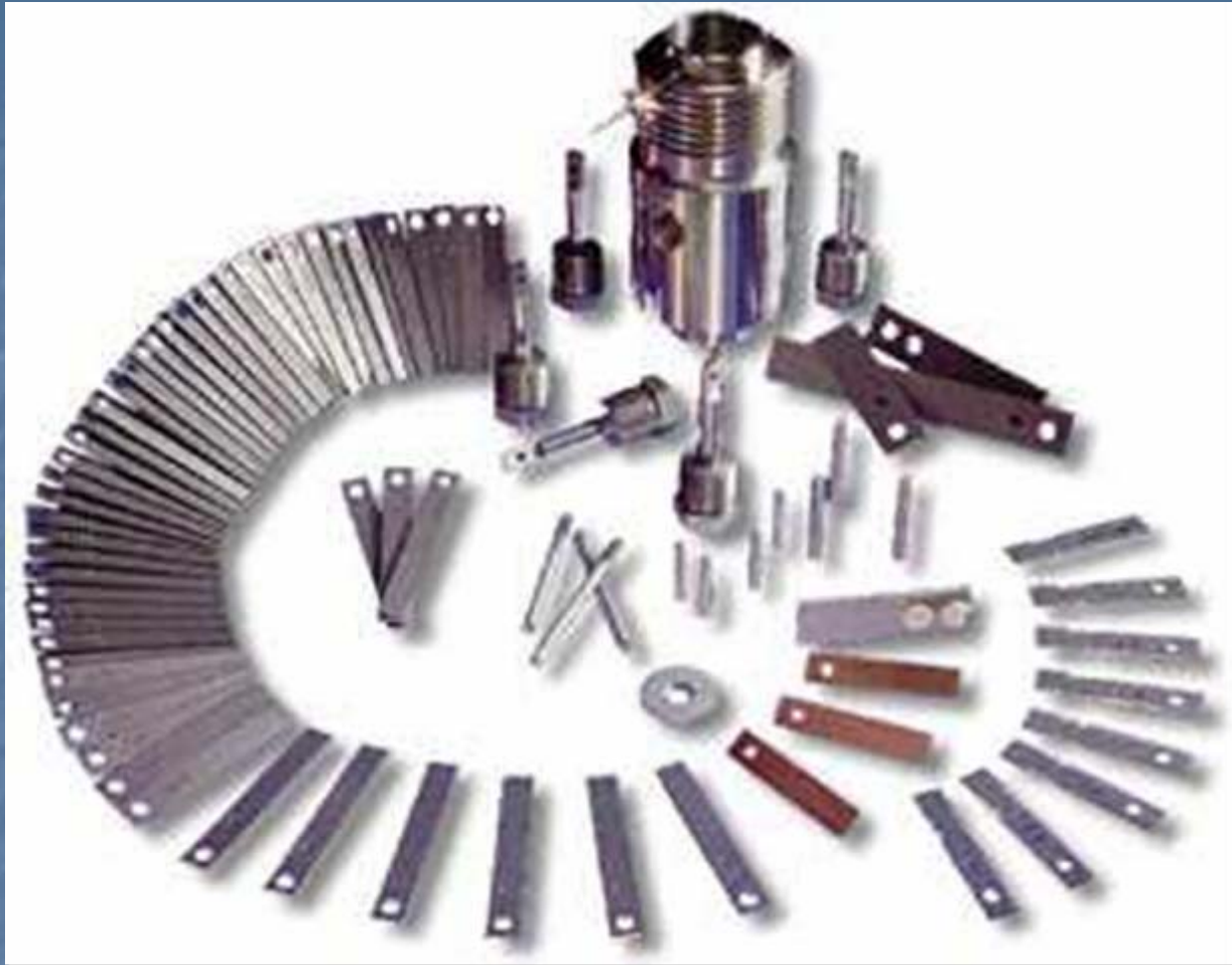
Type of test coupons that are used for corrosion testing
