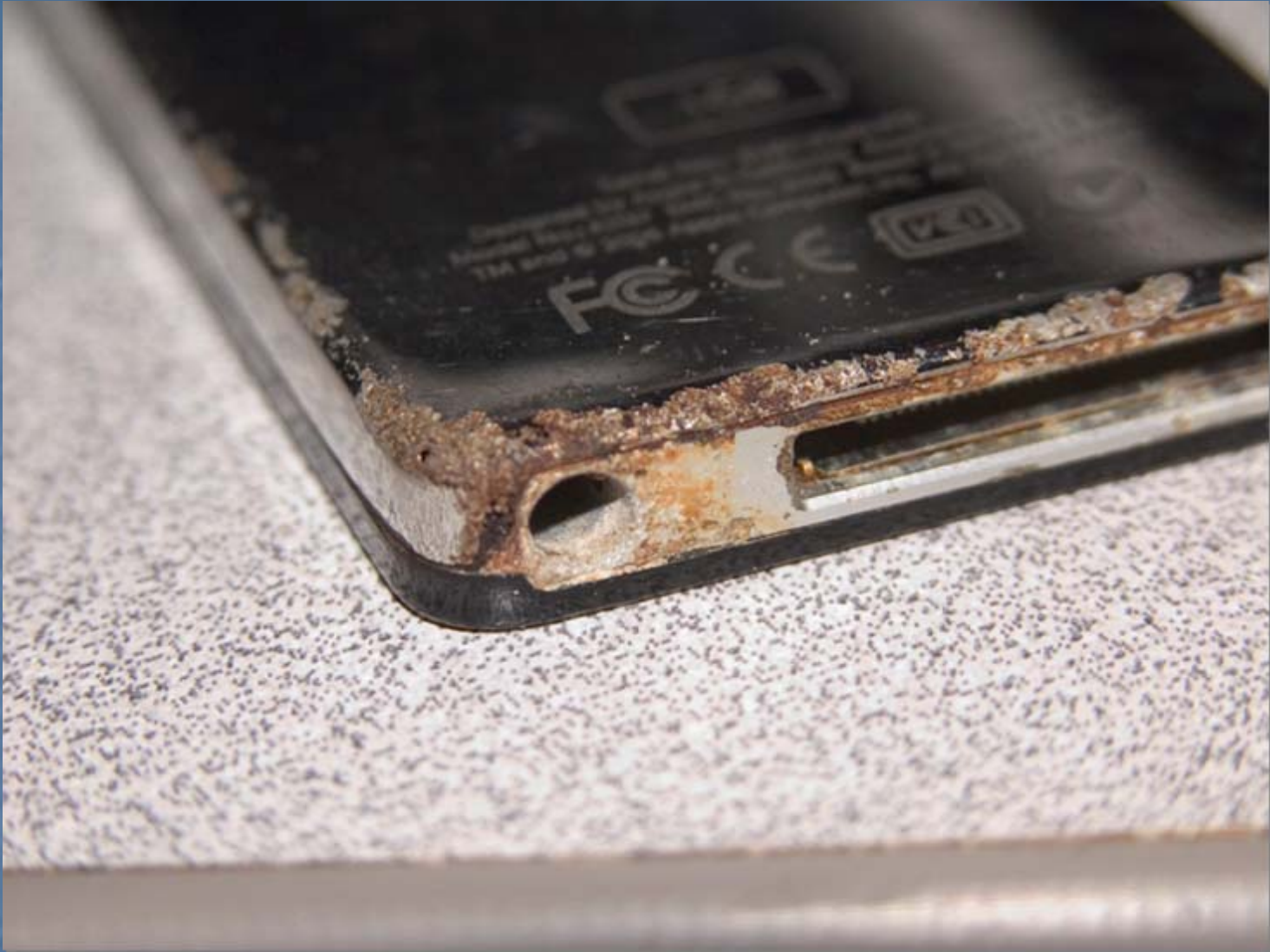
Corrosion of ipod nano
