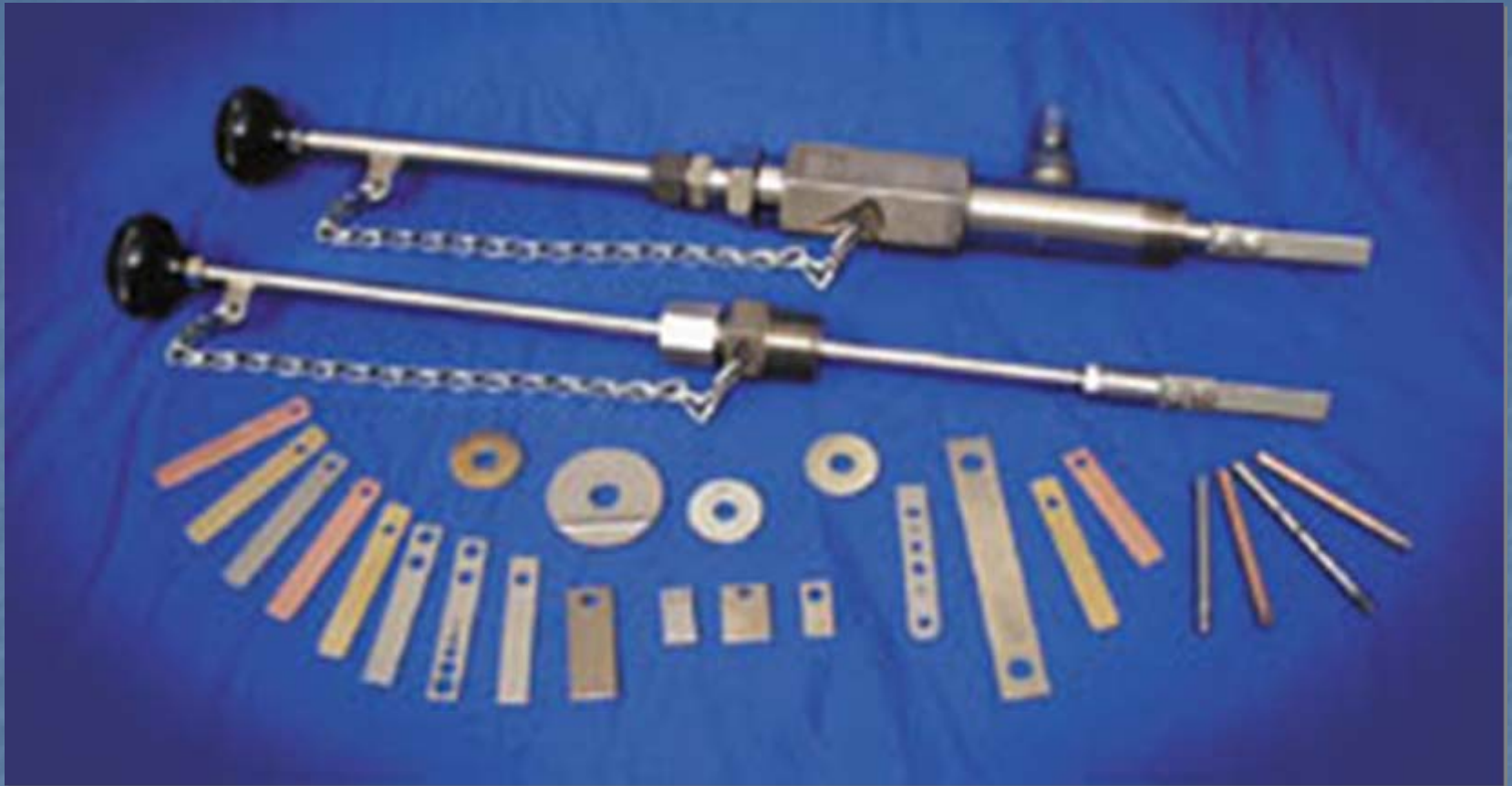
Type of test coupons that are used for corrosion testing
