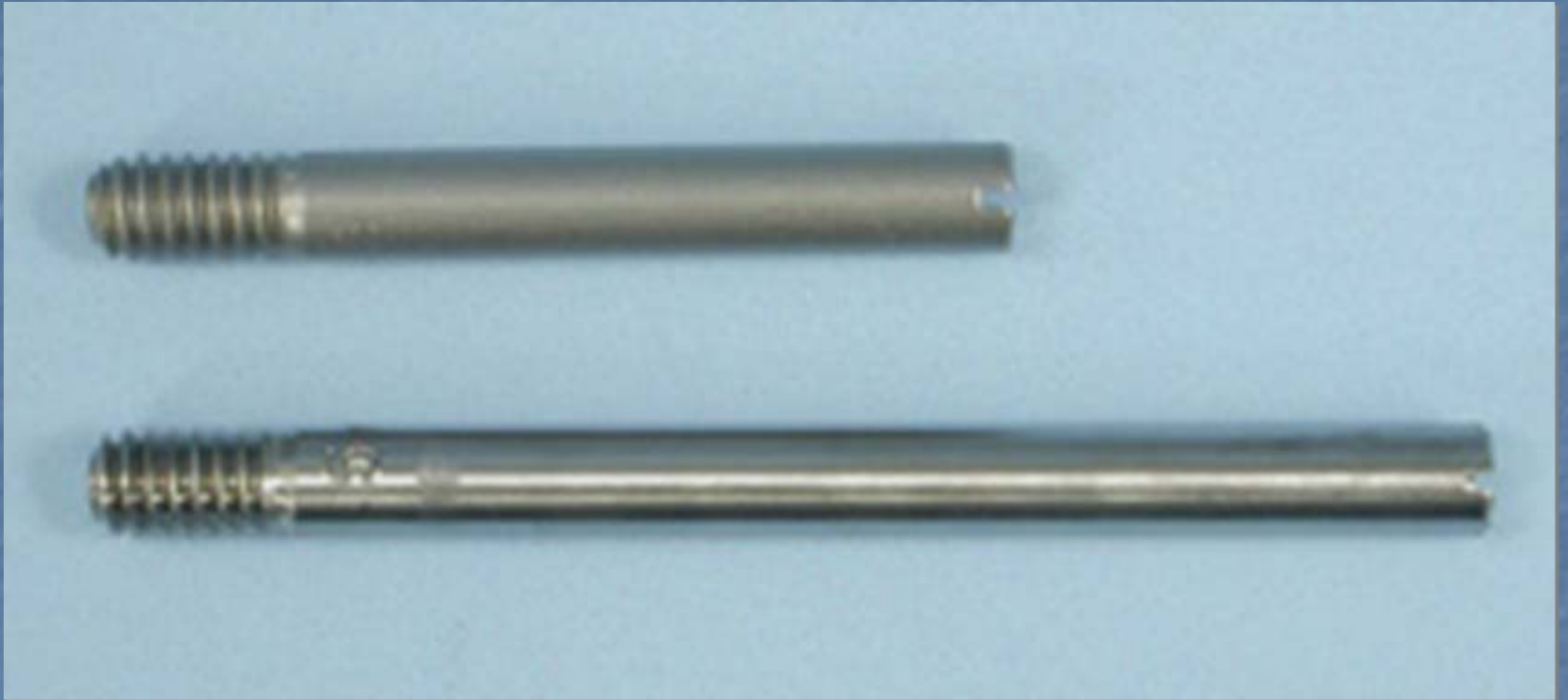
Cylindrical test coupons that are used for corrosion testing
