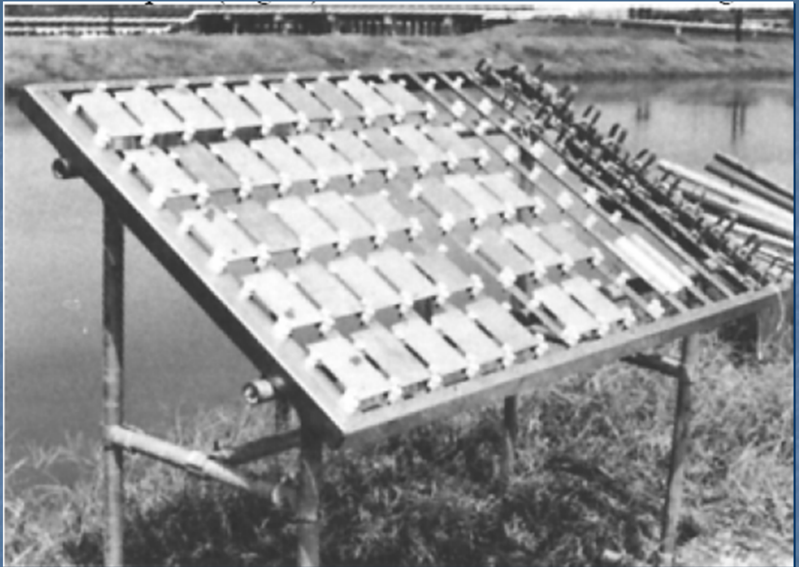
Atmospheric-corrosion test rack
