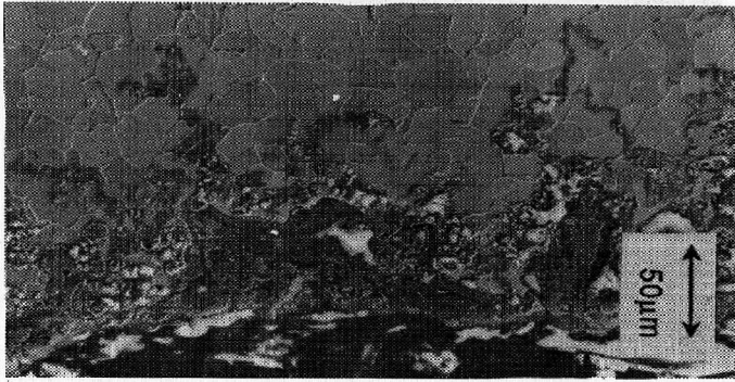
Fig. II.1 : Corrosion product layer on the inner tube surface, protruding into the metal substrate, shown on a section taken across the tube width
