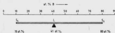
Fig. 7 : Lever for ascertaining phase proportions
