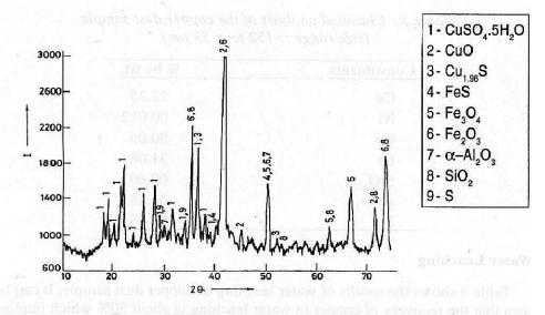
Fig. 1 : XRD pattern of copper dust sample.
