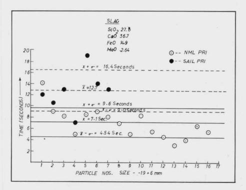
Fig.3 : Average melting time (x) and standard deviation of NML and SAIL sponge iron in acidic slag at 1300 °C in medium frequency coreless induction furnace
