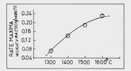
Fig.7 : Variation of the rate maxima with increasing tempeature of molten pool in induction furnace
