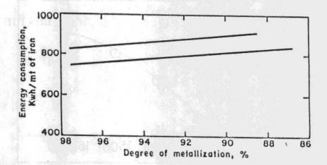
Fig. 9 : Effect of the degree of reduction of DRI on the energy consumption during batch melting in a coreless induction furnace
