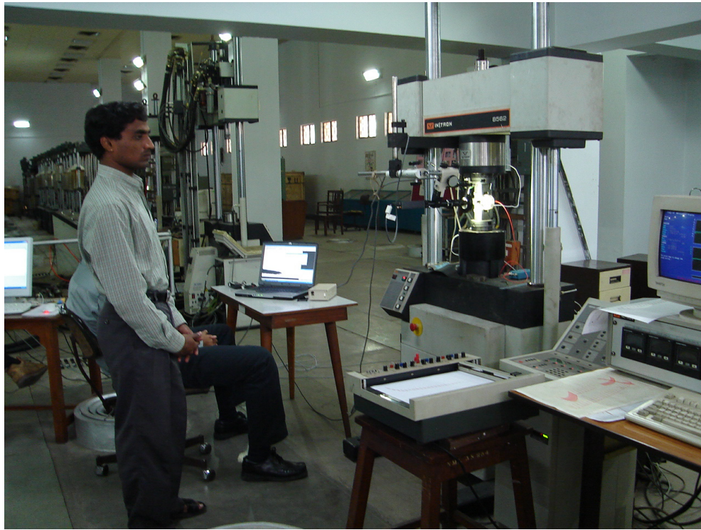
Figure 1 (a) : ROMS set-up being used for crack tip monitoring
