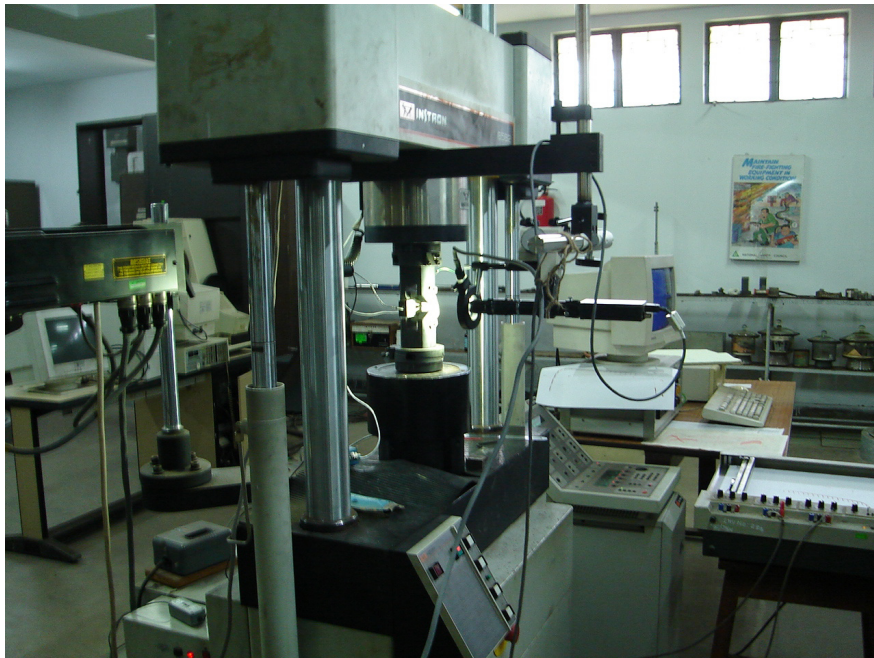
Figure 1 (b) : ROMS set-up with CCD camera attached with the servohydraulic machine
