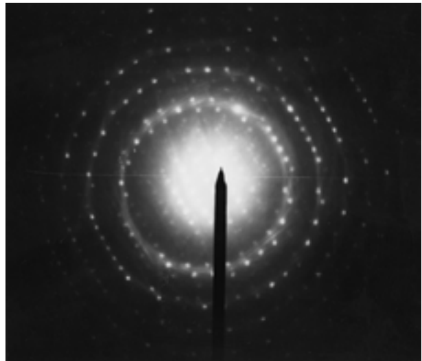
Fig. 3. SAD pattern of as-plated electroless Ni–P– \text{Si}_3\text{N}_4 composite coating. (Adapted from Balaraju [19].)
