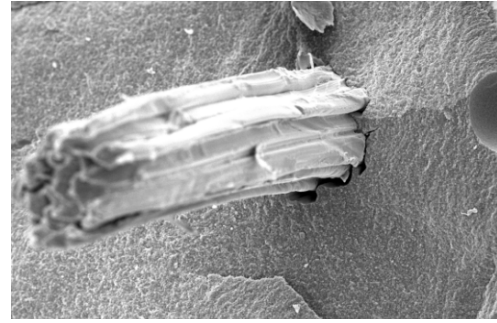
Figure 2. Scanning electron microscope (SEM) of Bombyx mori silk-fiber in FRC fracture surface (magnitude 50 µm)
