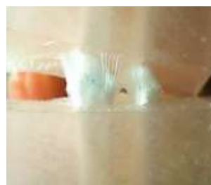
Figure 2. Macro fracture photos on the test rod with the addition of e-glass fiber. Fracture occurs only on resin acrylic.
