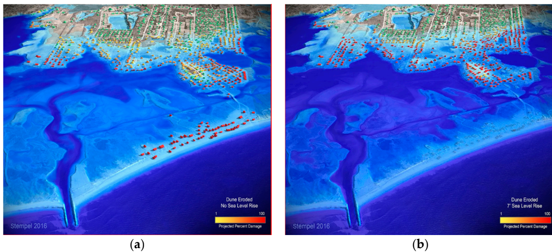
Figure 4. Three-dimensional visualization of the predicted damage by structure for 100 y and no SLR (a) and 100 y plus 7ft of SLR (b), dunes eroded [5] (personal communication, with the permission from Peter Stempel, 2016).
