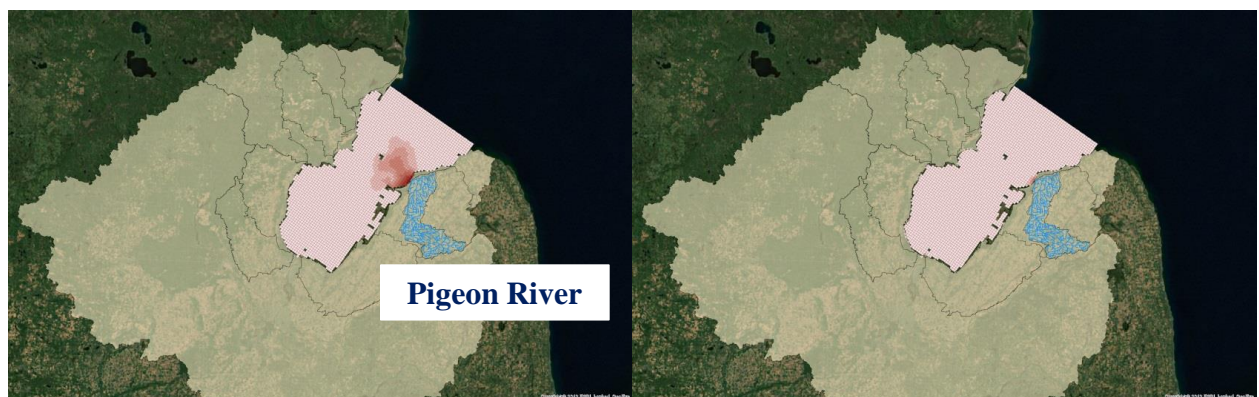
Figure 2.16. Relative contribution of Pigeon River to each 1km model grid cell. (left: cell contribution with only Pigeon River inflow; right: cell contribution with all tributary inflows.)
