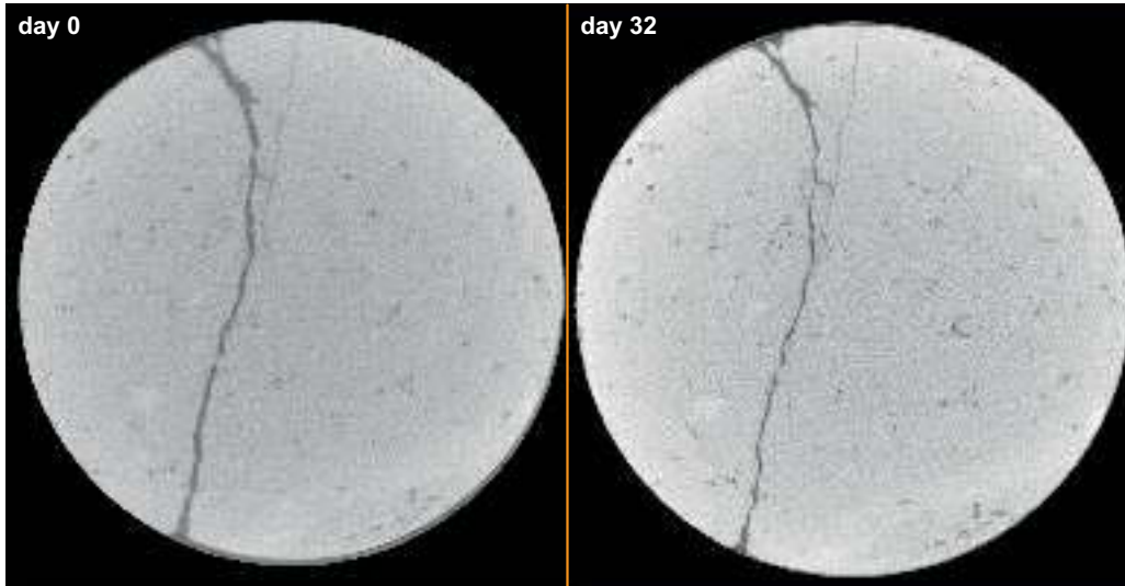
Figure 4.6: X-ray tomography scan of the 95°C run, showing no narrowing of pores between start (left) and right (end) of the experiment. The top images represent a top view; bottom images are cut at the red line and viewed from the right (see arrow). Here the reacted basalt shows the formation of a new fracture.
